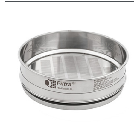
Stainless steel sieve with oval perforated plate (for cereals, ISO 5223).
