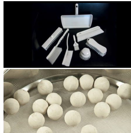
1. Cleaning brushes for sieves. 2. Food balls used to open the mesh of sieve.
